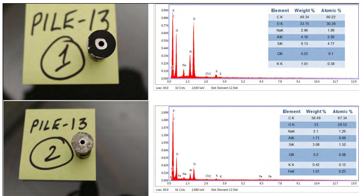
Figure 9: EDS data collected from the back side of the coating of the test dollies 1 and 2.
