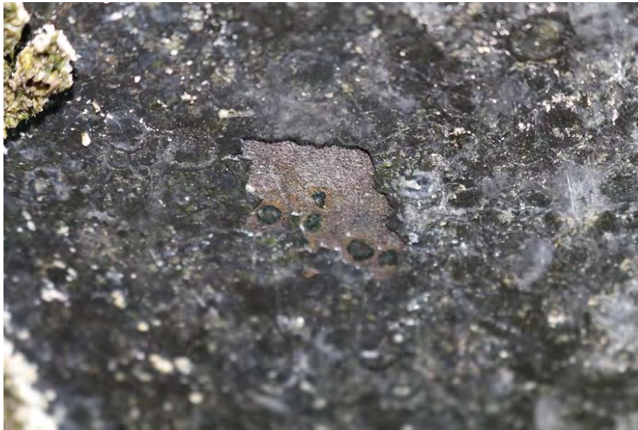
Figure 8: Photograph showing that the steel surface under the coating blisters is free from accelerated corrosion. Magnetite (black spots) can be clearly seen.
