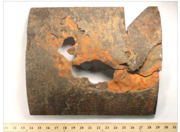
Figure 14: Photograph showing the holes and other areas of corrosion in the bottom side of the 16-inch diameter pipe.
