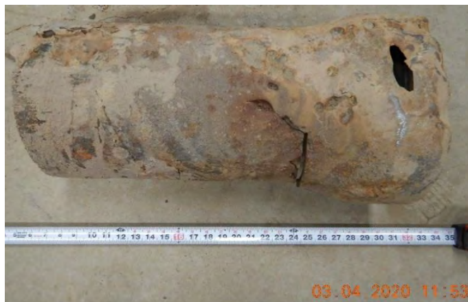
Figure 17: Photograph showing the perforation and some deep pits around the perforation in the as-received pipe section.
