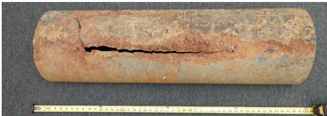
Figure 2: Photographs showing the failed watermain pipe section.
