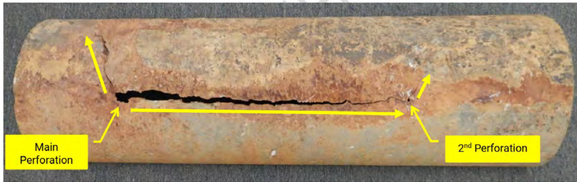
Figure 3: Figure 2 is retouched for better understanding to show the crack propagation. Main perforation and 2 nd perforation can be seen in the photograph.
