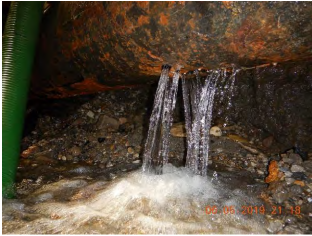
Figure 11: Photograph showing the water leakage from the bottom of the 16-inch diameter failed water pipe.
