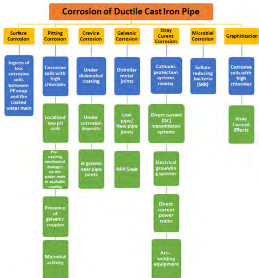
Figure 1: Photograph showing possible causes of external corrosion of DI pipe.
