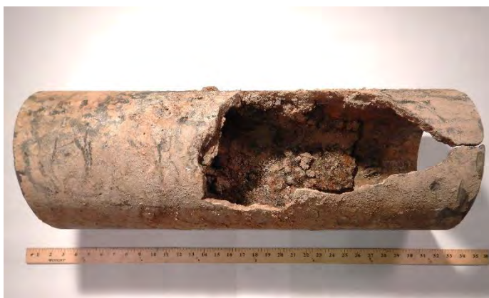
Figure 25: Photograph showing the pipe section cut from the failed location of the 8-inch diameter failed water pipe. Tubercles at the internal surface of the water pipe are clearly visible.
