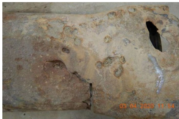
Figure 18: Photograph showing the perforation and some deep pits around the perforation in the as-received pipe section.
