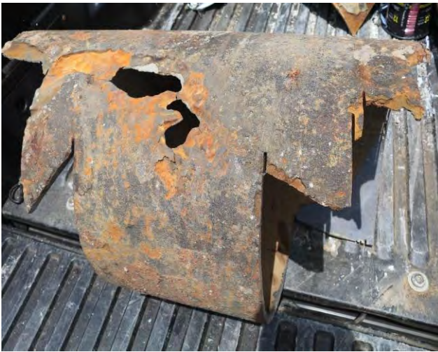
Figure 13: Photograph showing the holes in the bottom side of the 16-inch diameter pipe.
