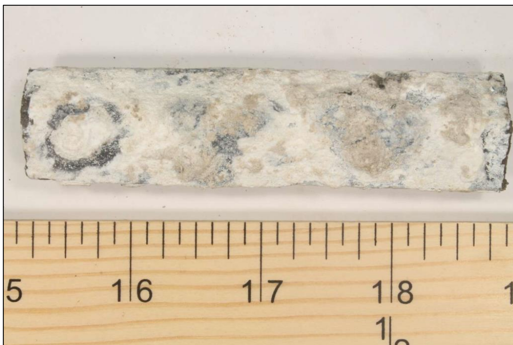
Figure 5: Photograph of corroded zinc ribbon from corrosive soil in Western United States.
