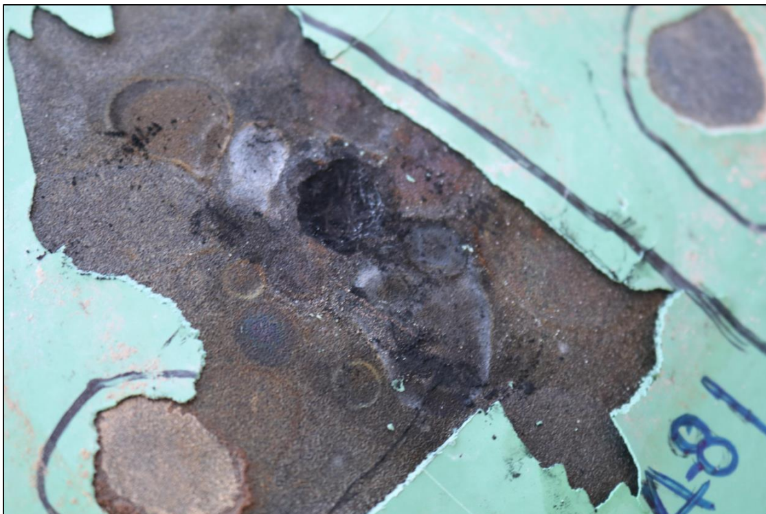
Figure 2: Close-up photograph of AC stray current corrosion penetrating deep into the pipe wall.
