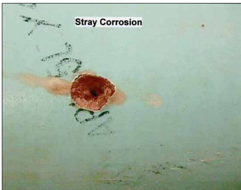
Figure 3: Photograph of localized corrosion due to DC stray current. The appearance of DC stray current corrosion is similar to that AC stray current corrosion. Site testing is required to distinguish between AC or DC stray current corrosion damage.
