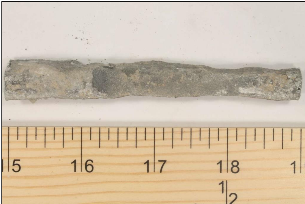
Figure 6: Photograph of corroded zinc ribbon from corrosive soil in Western United States – corrosion products removed for analysis.
