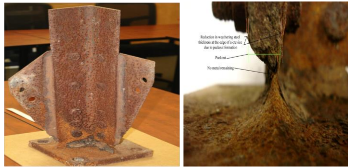
Figure 5 - Photographs exhibiting buildup of Pak-out and loss in thickness of load bearing member (photo on-right hand side)
