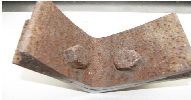
Figure 9 - Pack out Piece that was used for FEA Analysis
