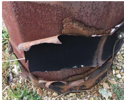
Figure 3 – Example of dis-bonded coating and expansive corrosion products in the crevice formed between polyurethane coating and weathering steel substrate (Source: Author(s))
