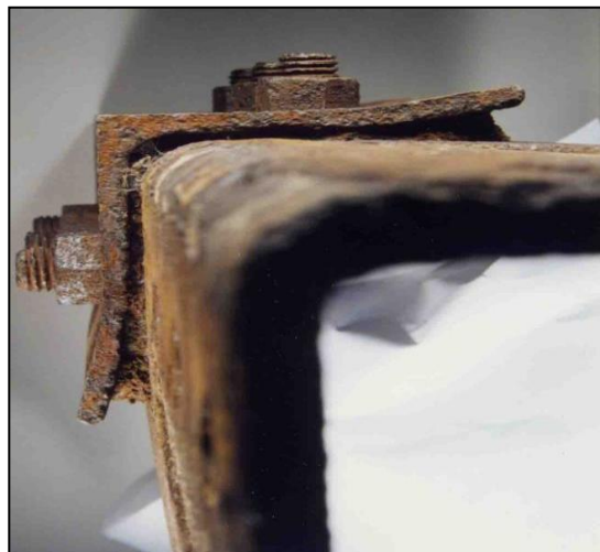
Figure 6 - Pack-out formation on bolted joints
