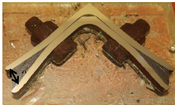
Figure 10 - Joint Cross Section showing porosity in pack-out.
