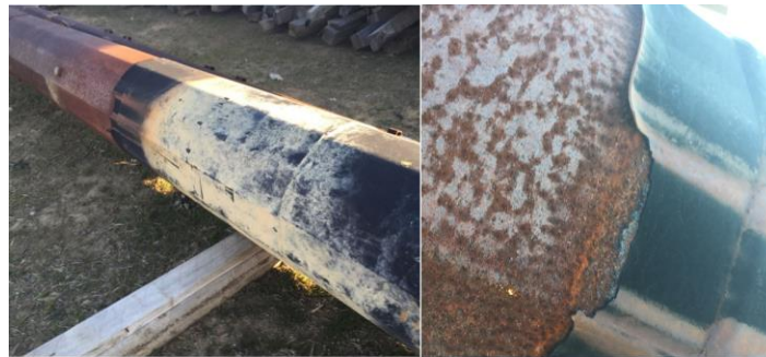
Figure 2 – Embedded 2 nd generation weathering steel pole removed from service after 16 years. The coating is in excellent condition above and below grade, with less than an inch of adhesion loss at the coating interface. (Source: Author(s))
