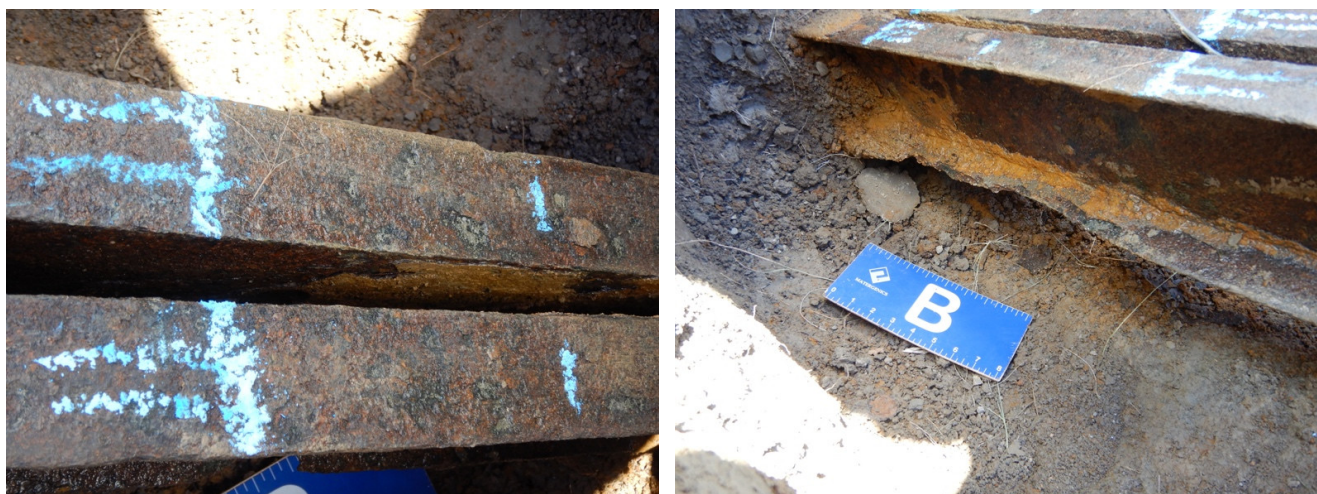
Figure 7. Example of visual factor = 4 or anchor shafts under a severe corrosivity level
