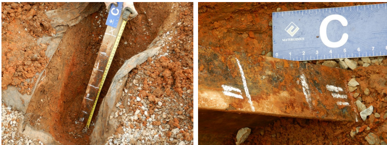
Figure 6. Example of visual factor = 3 or anchor shafts under a high corrosivity level
