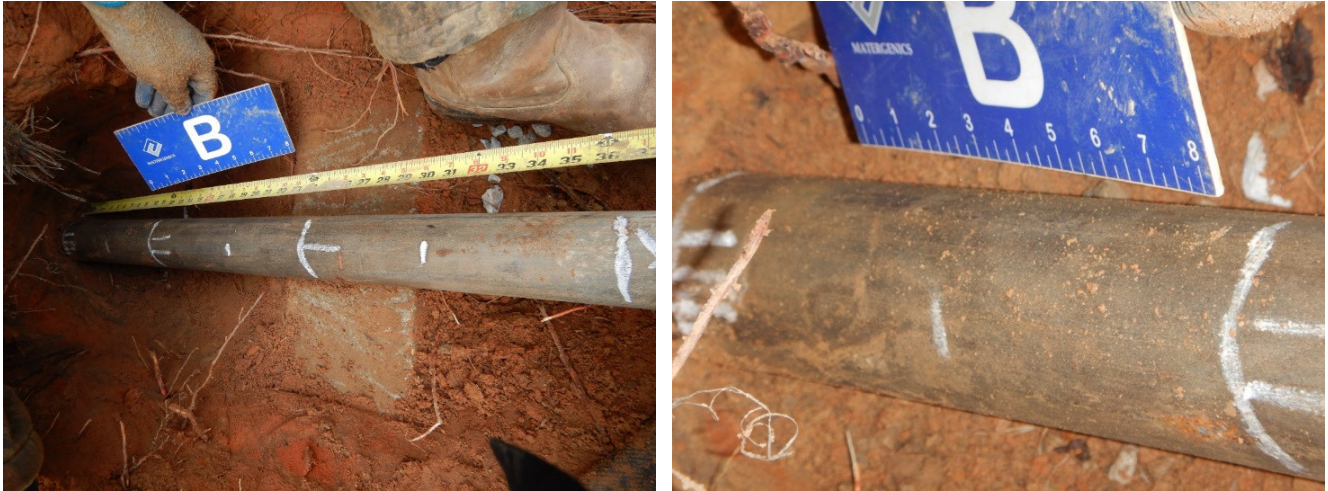
Figure 4. Example of visual factor = 1 or anchor shafts under a mild corrosivity level
