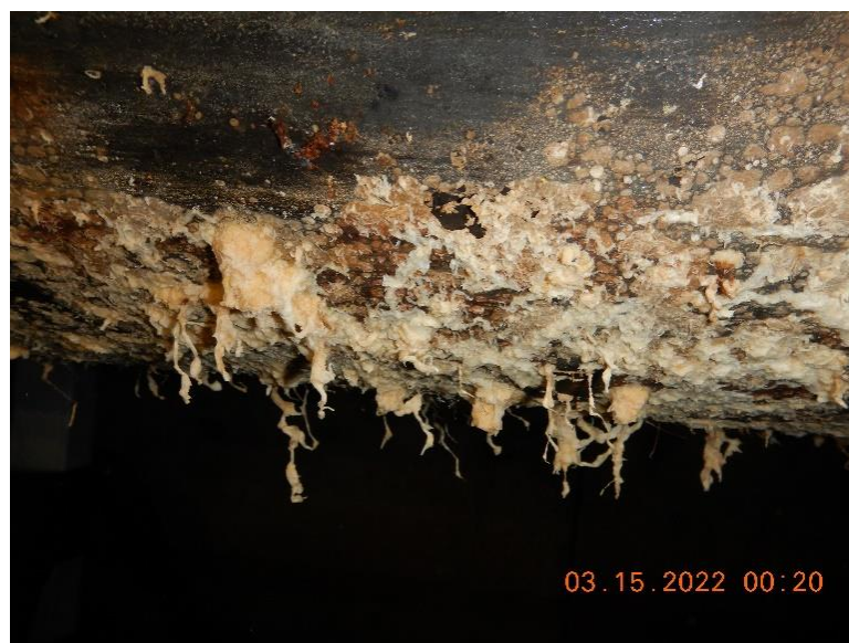
Figure 17: Photograph showing white deposit build-up on the pipe at the 6 O' clock position.
