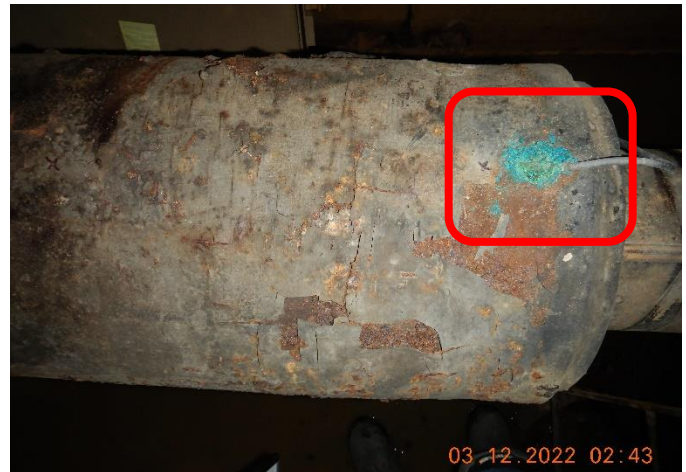
Figure 8: Photograph showing corrosion of the Cad weld connection.
