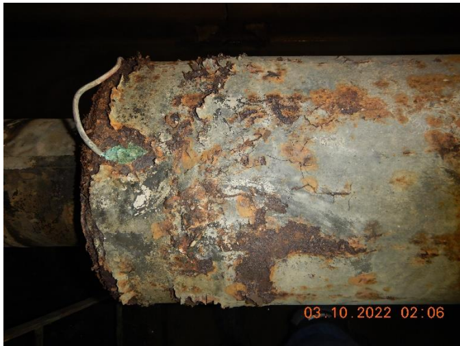
Figure 5: Photograph showing coating deterioration and corrosion of the underlying steel pipe casing.
