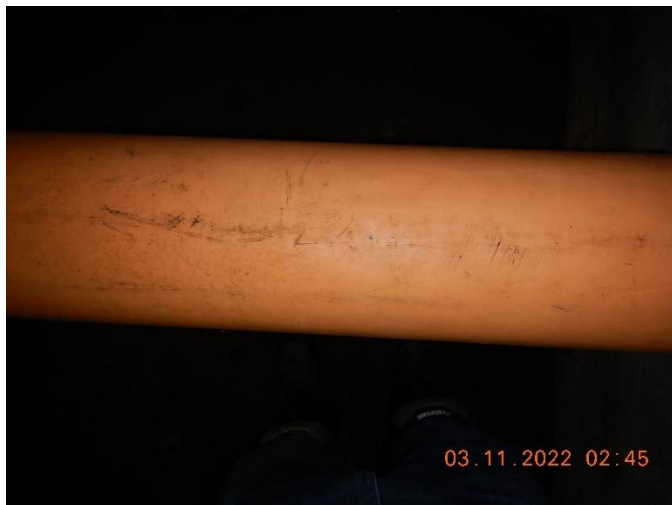
Figure 9: Photograph showing the condition of the coating on the carrier pipe.
