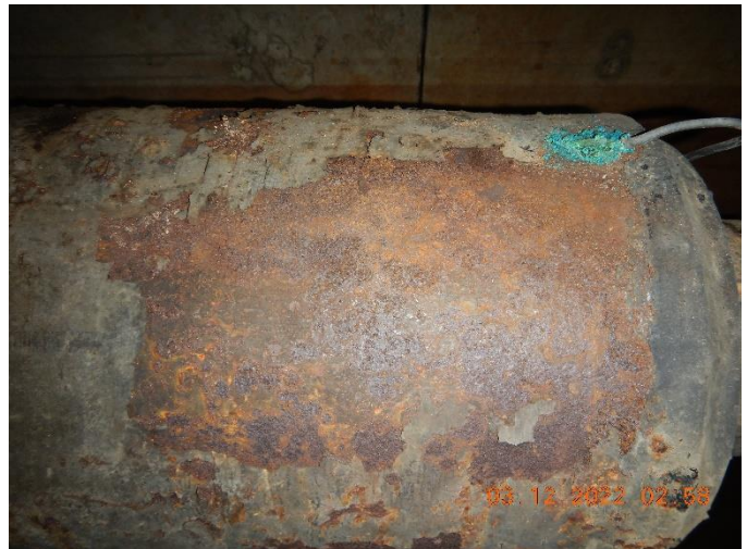
Figure 6: Photograph showing coating deterioration and corrosion of another steel pipe casing.
