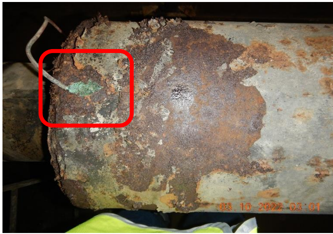
Figure 7: Photograph showing corrosion of the Cad weld connection.
