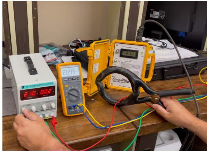
Figure 2: Photograph taken during the verification of swain meter.
