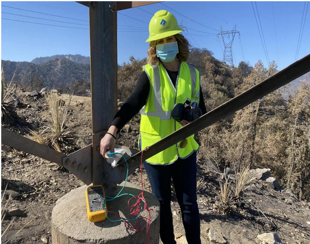
Figure 8: Measurement of corrosion potential will indicate the corrosion activity on galvanized members.
