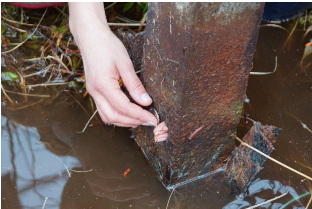
Figure 5 a): Corrosion Perforation in Corrosive Water
