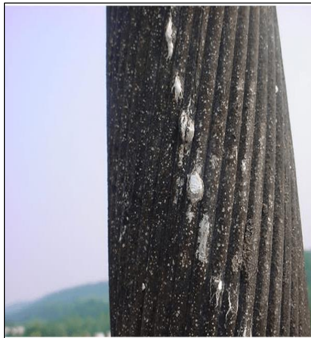
Figure 14: In another case zinc was observed due to high temperature exposure above 850 F (454°C). No such melting observed in this case.
