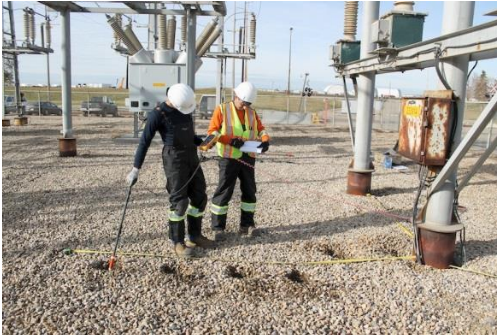
Figure 4: Corrosion crew performing corrosion risk assessment in a substation.
