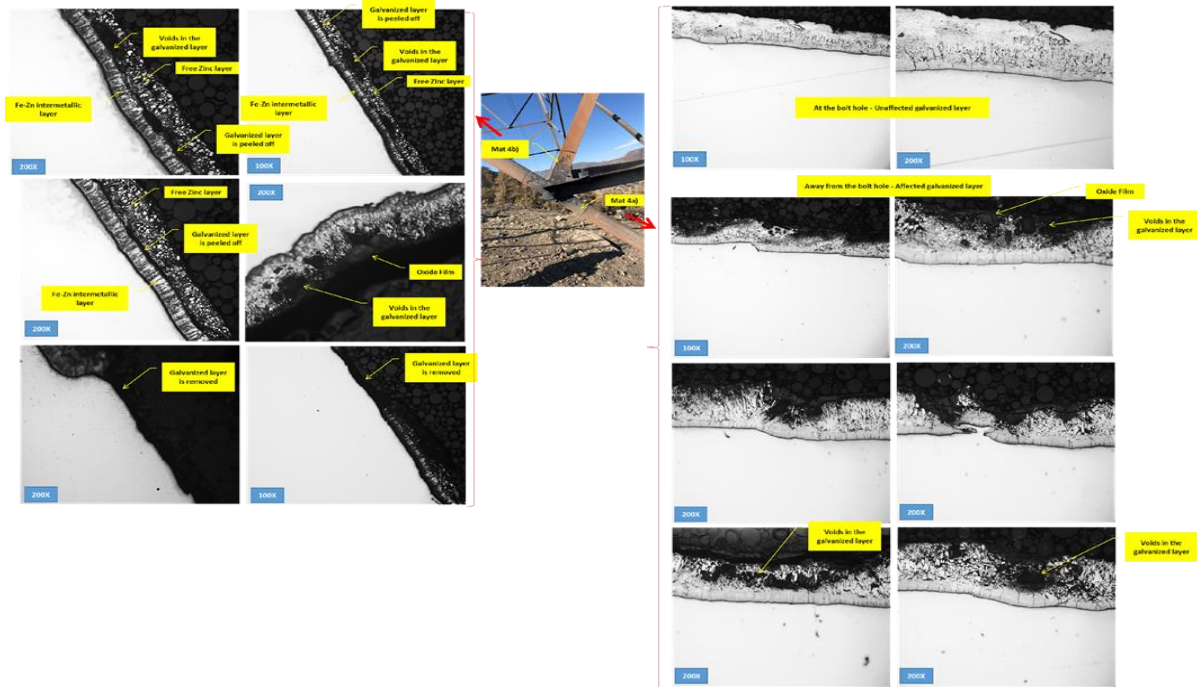
Figure 2: Cross sections of galvanized members exposed to wildfire and the damage observed indicating oxidation and delamination of galvanized layer due to temperature raise above 350F (177°C) 1 .
