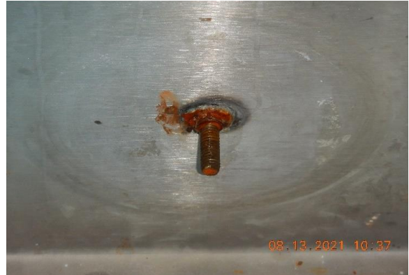
Figure 26: Photograph showing the condition of SS bolt welded to the frame. Anode 22 is bolted at this location. Presence of rust can be clearly seen.
