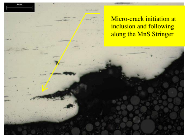
Figure 3: Photomicrograph taken at the reduced diameter showing micro-crack initiation at inclusion and the microcrack is following along the MnS Stringer. Magnification: 100X.
