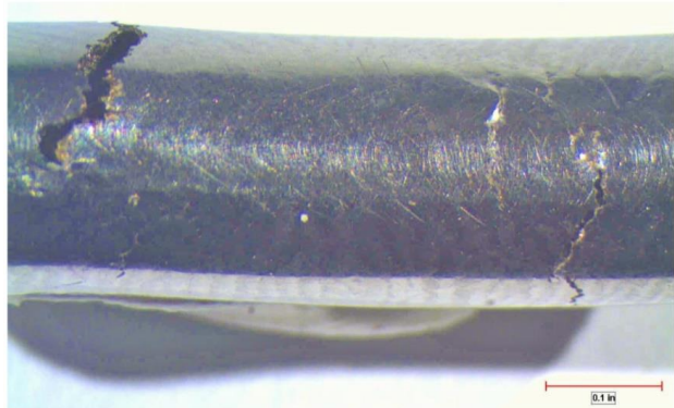
Figure 28: Closer view of the region highlighted in the red box, as shown in figure 27, showing numerous additional cracks other than the visible crack. 7X
