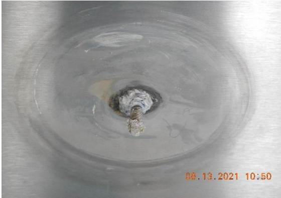
Figure 25: Photograph showing the condition of SS bolt welded to the frame. Anode 6 is bolted at this location. White deposits can be clearly seen.
