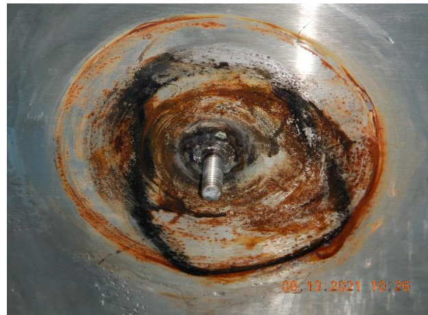
Figure 24: Photograph showing the condition of SS frame where anode 3 was in contact with the frame. Corrosion of SS frame in contact with the rubber of the anode 3 can be clearly seen.
