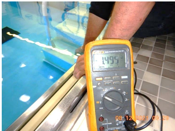
Figure 17: Photograph showing the anode B-to-water potential value.
