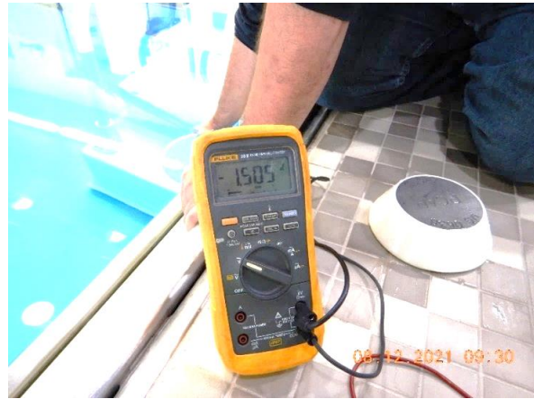
Figure 16: Photograph showing the anode A-to-water potential value.
