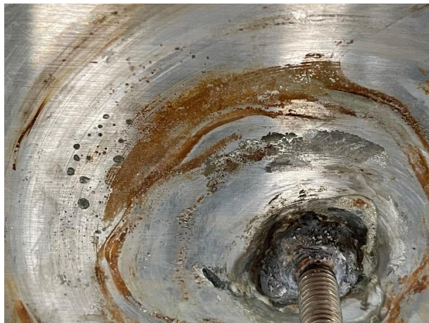
Figure 23: Photograph showing the condition of SS frame where anode 4 was in contact with the frame. Corrosion of SS frame in contact with the rubber of the anode 4 can be clearly seen.
