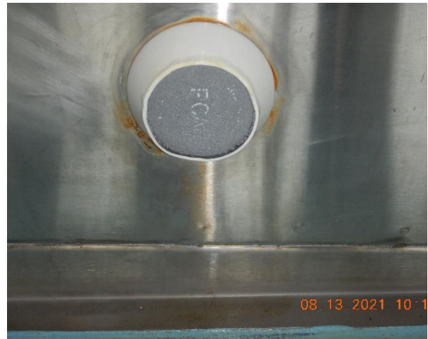
Figure 22: Photograph showing the condition of anode 4. Corrosion of SS frame behind the anode 4 can be clearly seen.
