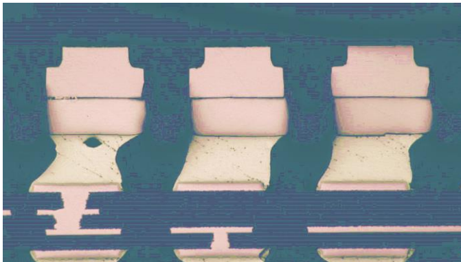
Figure 11: Photomicrograph of the fourth, fifth, and sixth pins from the brand-new charger cable from the original manufacturer. Magnification: 50X
