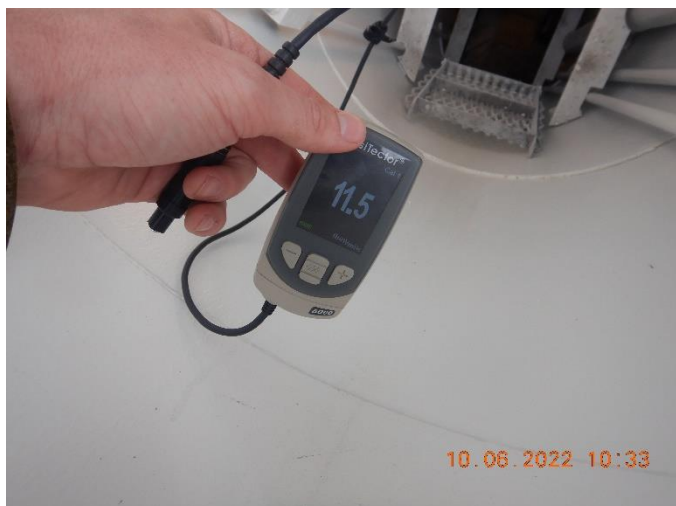
Figure 13: Photograph showing the coating thickness (in mils) of entrance tube of the pump station 5.
