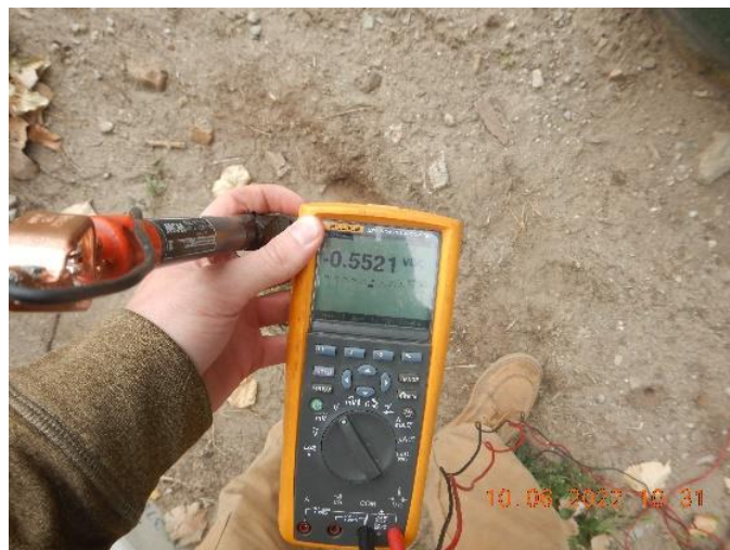
Figure 16: Photograph showing the structure-to-soil ON potential of the pump station 5.
