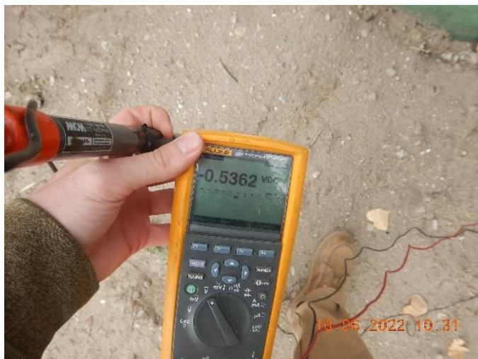
Figure 15: Photograph showing the structure-to-soil ON potential of the pump station 5.
