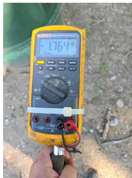
Figure 23: Photograph showing the structure-to-soil ON potential of the pump station 5.
