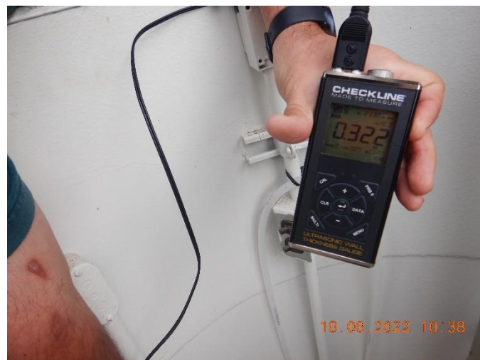
Figure 14: Photograph showing the wall thickness (in inches) of entrance tube of the pump station 5.
