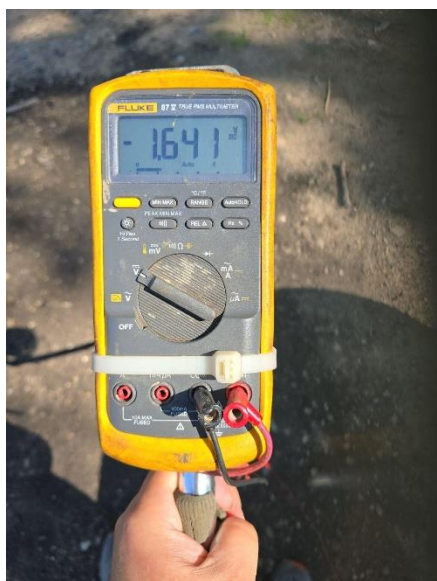
Figure 22: Photograph showing the structure-to-soil ON potential of the pump station 5.
