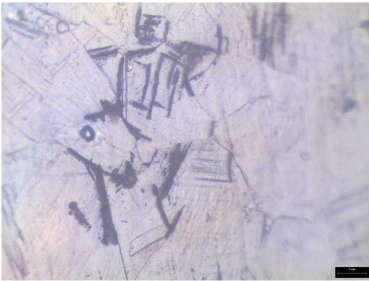
Figure 29: Photomicrograph showing cracks in the examined area. Interestingly, the cracks were confined only to the regions with prior cold worked grains. The cracks were similar to stress relaxation cracking. Magnification: 200X
