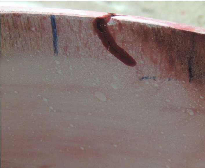
Figure 3: DPT of the as received flange on the inner surface.
